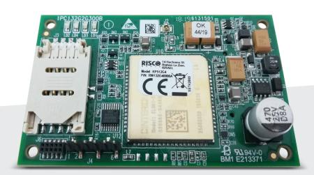
The 4G Communication Module is a plug-in module, enabling RISCO Control Panels to communicate via 4G/3G networks for reporting, control and remote programming. It can be used as the primary communication or as backup for the IP and Wi-Fi communication module. The module supports the SIA/IP, SIA and Contact ID reporting formats.
